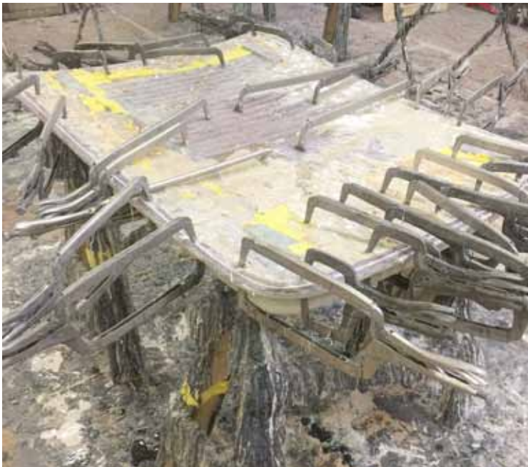
Clamps everywhere to hold this hood while the glass cures overnight.
