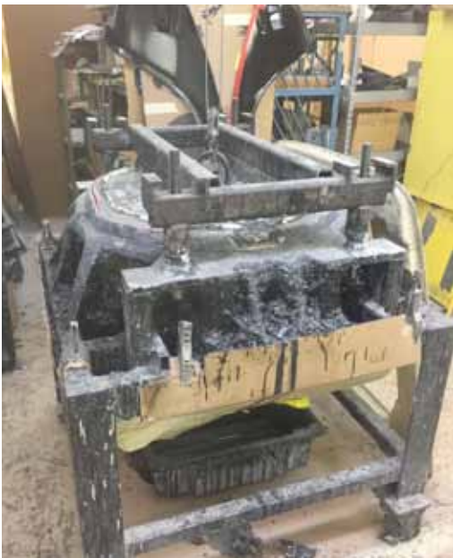
C-2 Spare Tire carrier in the mold
