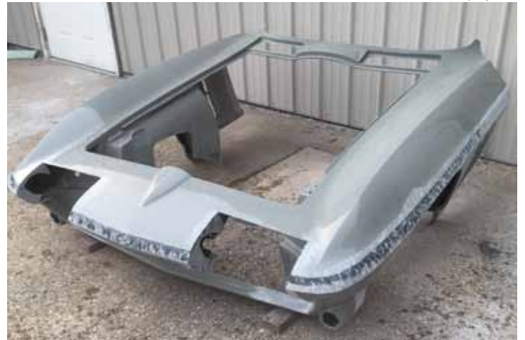
C-2 complete front clump with inner fender panels, assembled and ready to ship out
