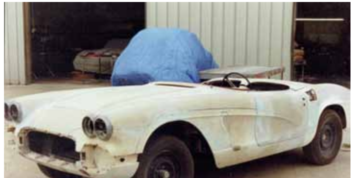
The rear wheel openings had been flared and we put on new panels to restore the original body lines.
