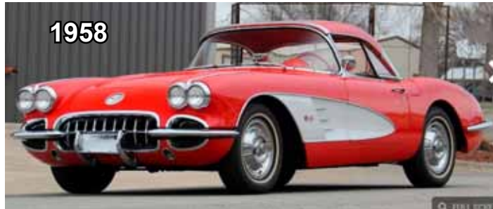
Signet Red with White coves. Red interior. Color-keyed removable hardtop 283 CI V-8 engine. Carter 4-barrel carburetor: Aluminum intake. Finned aluminum valve covers. 4-speed manual transmission.
