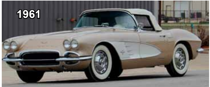
Fawn Beige with White coves. Fawn interior. Beige soft top. 283/230 HP V-8 engine with a 4-barrel carburetor: 4-speed manual trans. First year the 4 round tail lights were incorporated.
