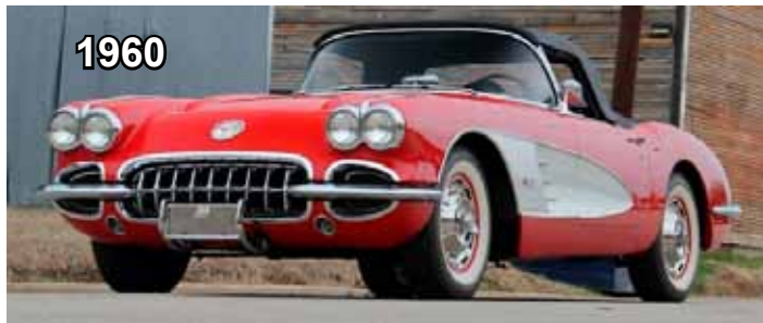
1 of 859 Corvettes produced with fuel injection for 1960. 283 CI V-8 engine. Rochester fuel injection unit. Finned Corvette script valve covers. 4-speed manual trans. Roman Red with White coves and a Black soft top. Black interior.
