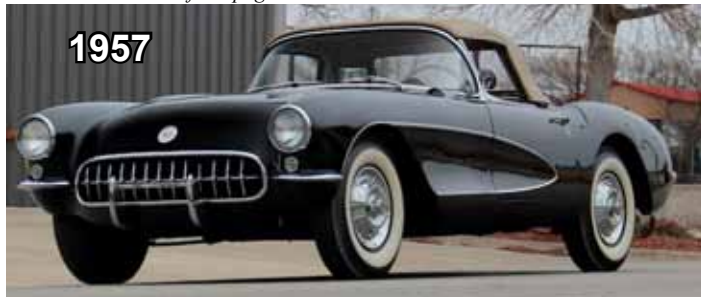
283/245 HP V-8 engine. Two 4-barrel carburetors. Powerglide trans. Onyx Black with a Beige folding top. Beige interior. 3-spoke competition steering wheel Updated pushbutton style radio with cassette.
