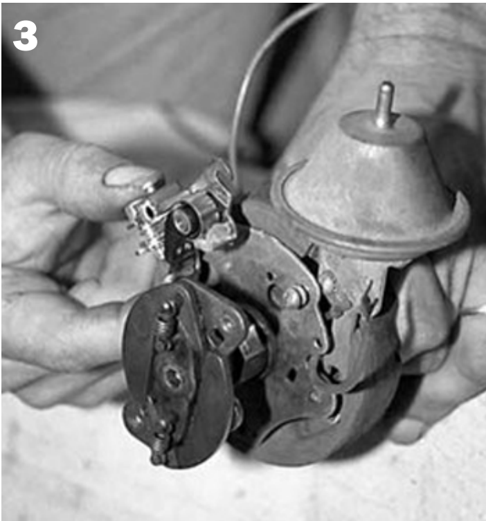
Remove the rotor, coil wire and condenser wire from the point assembly. Then remove the breaker points assembly. Keep the screws and washers, because you will reuse them.
