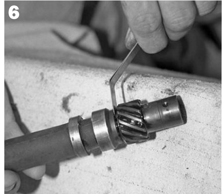
On Delco Corvette distributors, the shaft has a tendency to climb as the car is started and as the engine accelerates. This is due to the bevel of the gear on the distributor shaft and camshaft. If the clearance between the gear and the lower end of the distributor housing is too great, it may allow the clearance between the magnet ring and the module to become more than .100". When this happens, the engine will miss or not fire. Here we are checking the clearance and we found it to be too great.
