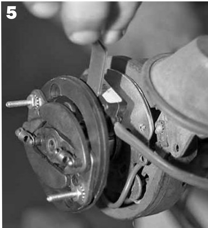
Install the magnet ring with the two threaded 6/32 studs. Keep the nuts and the two thick washers. Now check the air gap between the face of the magnet ring and the face of the Ignitor module. It should be not be less than .010" and not more than .040".
