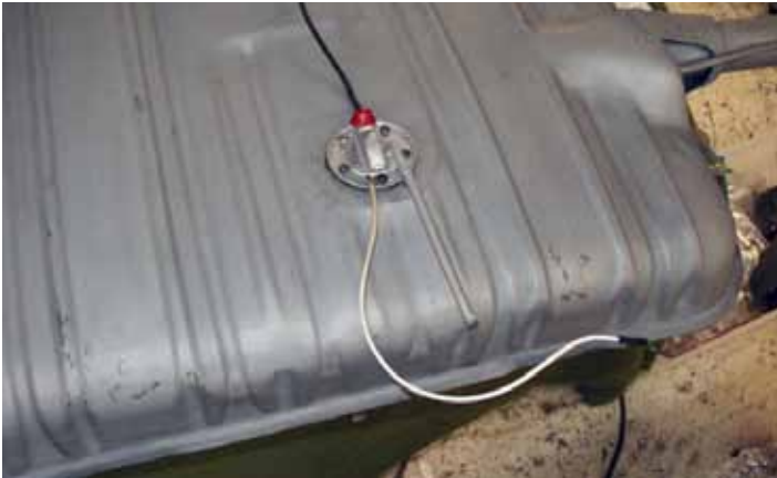
The white wire in this fuel gauge grounds the sender body directly to the frame.
