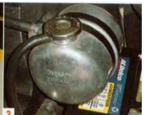
3 The Harrison aluminum expansion tank with the inlet and overflow at the top and the outlet at the bottom. Only fill half full when cold or it may puke coolant out the overflow during hot-soak.
