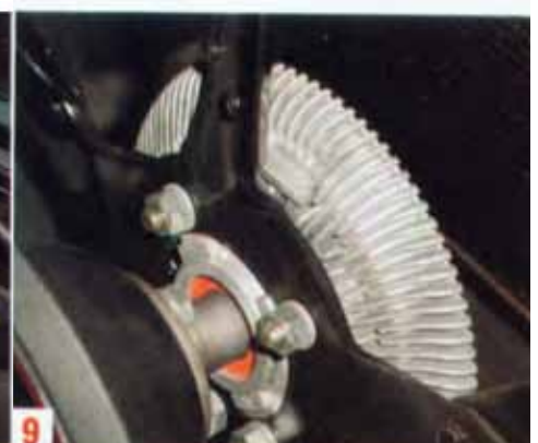
9 The thermo-modulated Corvette fan clutch is key to idle and low-speed airflow and far more efficient than any flex-fan. They can be rebuilt when not working properly.
