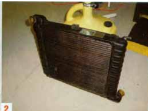
2 A typical look-alike copper/brass replacement radiator; note the rounded/stamped end tanks. These have about 30% less cooling capacity than the original Harrison aluminum radiator.
