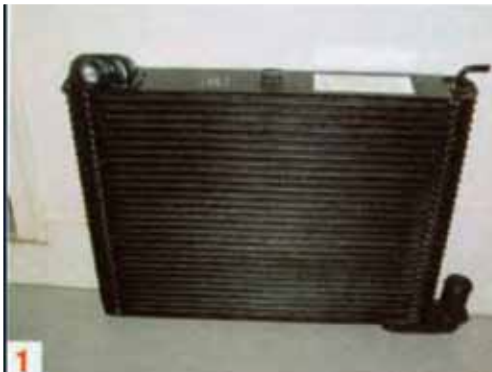
1 The extremely efficient Harrison stacked-plate aluminum radiator basic design was used from 1960-1972, and all versions are reproduced by Dewitts.
