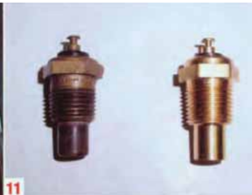
11 The original AC temp sending unit on the left, and a Wells TU5 replacement on the right; calibration of replacements is always suspect; check the gauge reading against an infra-red gun shot of the upper radiator hose.
