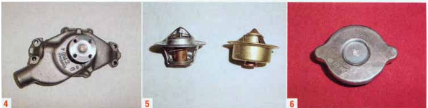
The stock Corvette water pump was designed and developed to meet the needs of the cooling system; you don't need a race water pump.
