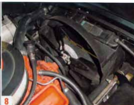
8 The fan, clutch, radiator and shroud are an engineered system; keep them as originally configured to maintain your Corvette's cooling airflow management.
