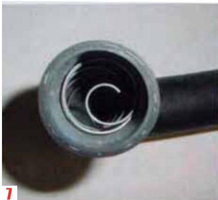
7 Original lower radiator hoses had this coiled steel wire reinforcement to prevent collapse. Modern hoses are made from better materials and generally don't need the wire to keep them open.
