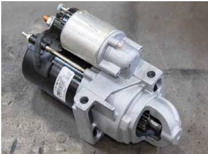
4. This Duralast gear reduction starter with staggered holes is typical of those used with large-diameter ring gears.
