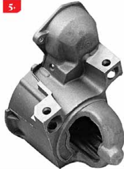
5. Starters using snouts with mounting holes straight across are compatible with small-diameter ring gears.
