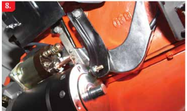
8. Here, a starter brace is shown in place. It attaches to the starter and a threaded hole in the block.
