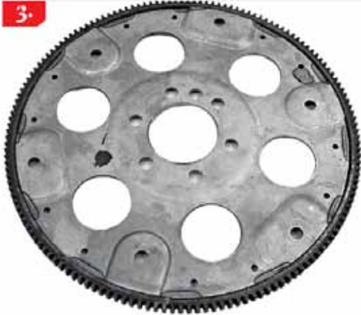
3. Chevrolet V-8s may be equipped with either 168- or 153-tooth ring gears. Each requires a specific starter.
