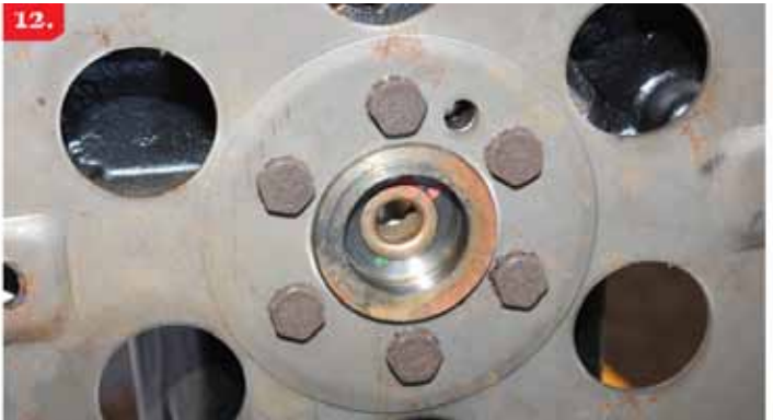
12. This crate engine came with a pilot bushing for a manual transmission, which in turn kept the converter from seating and warped the flexplate and caused the starter to make a ridiculous amount of noise.
