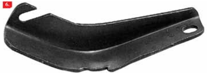
6. Direct-drive starters are heavy, and those with studs in the endplate require a brace to stabilize them.
