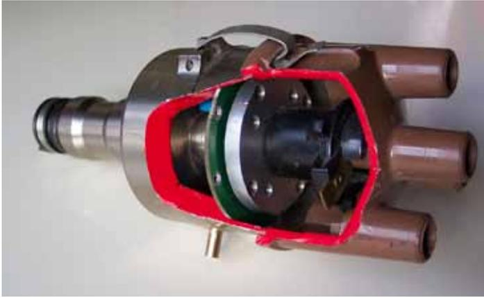
The 123 distributor provides both electronic triggering and electronic spark advance (no more weights and springs).
