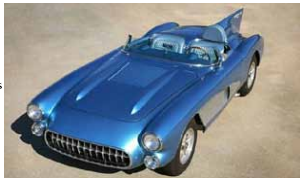
This 1956 SR-2 is unusual because it has an extended nose, headrest with fin and louvers in the hood.
