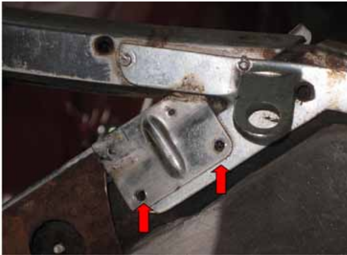
#3-4-5 connect the side rail to the rear window frame and are visible on the outside of the quarter window.
