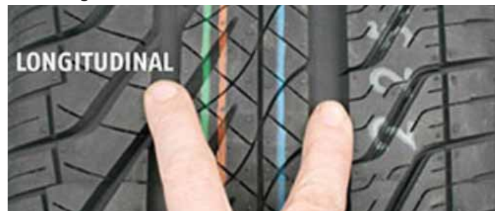
Longitudinal grooves in the tread allow for immediate water passage
