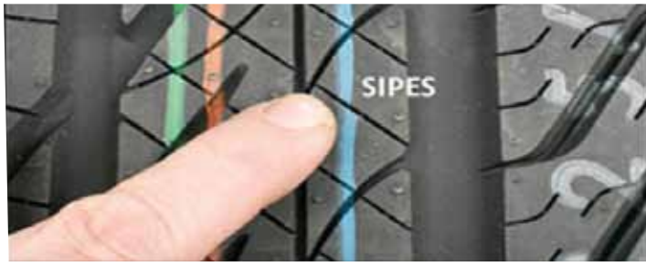
The smallest cuts in tread blocks are referred to as sipes. They provide added traction on wet or icy surfaces
