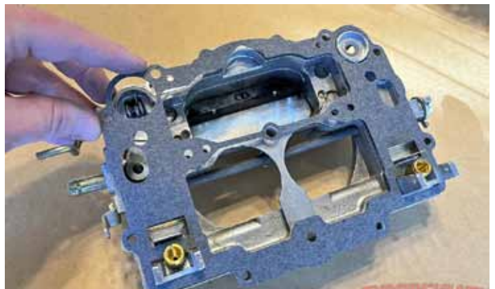
Moving to the top (air horn), we installed the new brass seats (with supplied washers) for the needle-and-seat assemblies, plus a new gasket to seal the air horn to the main body.
