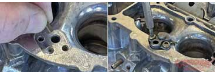
A new pump discharge ball, weight, and gasket were installed before screwing the cleaned pump jet housing back into place.
